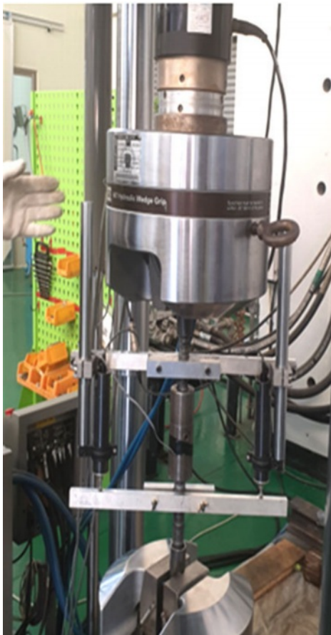
<High stress cyclic strength test>
